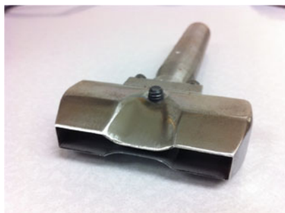
Fig. 2. ASTM dog bone punch (D-638-V) and the dimensions
